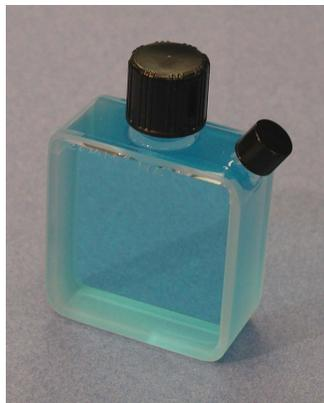
If you would like to bleed sample from a process line and/or pump liquid directly into and out of the transmission cell while it is situated in the instrument, you may wish to use a flow-through transmission cell like the one shown below.
