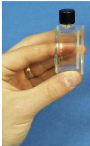
For hazardous or volatile liquids, you may wish to use a screw-top transmission cell rather than an open one. A 20-mm screw-top cell is shown below.
