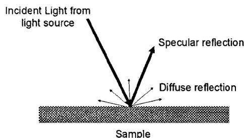
Sphere instruments used in the reflectance specular included mode minimize the effect of differences in gloss, texture, and directionality. For example, if two equally pigmented samples, one glossy and one matte, were measured on a sphere instrument, the readings would indicate that they are roughly equivalent in pigment color, even if they do not appear to be the same visually.
