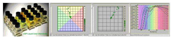
EP - European Pharmacopoeia Color is a similar visual liquid color scale used in the pharmaceutical industry. It consists of 3 primary color standard solutions (yellow, red and blue) that are combined with hydrochloric acid to make 5 standard color solutions - B (brown), BY (brownish-yellow), Y (yellow), GY (greenish-yellow) and R (red) that are subsequently diluted with hydrochloric acid (10 mg/l) to make 37 reference EP liquid color standards - 9B, 7BY, 7Y, 7GY and 7R.
