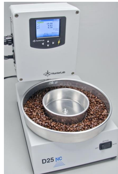
Figure 3: D25 NC (Non-Contact) measuring port down on both ground coffee and beans.
