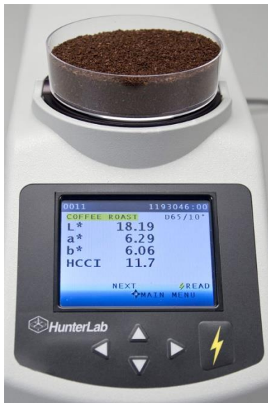
Figure 2: ColorFlex EZ Coffee measuring roast coffee color though the bottom of a clear plastic dish.
