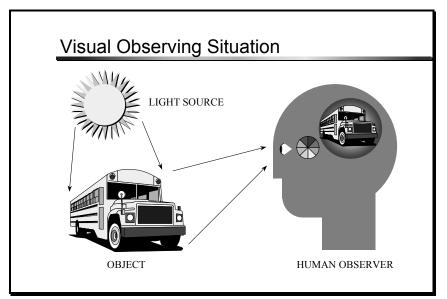
Color may be evaluated subjectively (visually) or it may be evaluated objectively, as with a spectrophotometer or colorimeter. In order for color to be quantified objectively, all three components of the visual observing situation must be taken into account.
