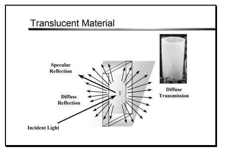
When examining or measuring an object for color and appearance, it is important to categorize it as an opaque nonmetal, opaque metal, transparent material, or translucent material. The category of an object gives important clues about how it should be measured.
