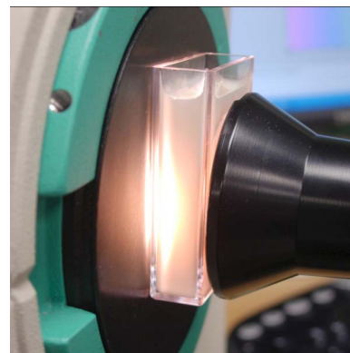
10-mm Acrylic Cell used to measure color of near-opaque liquid in RSEX reflectance
