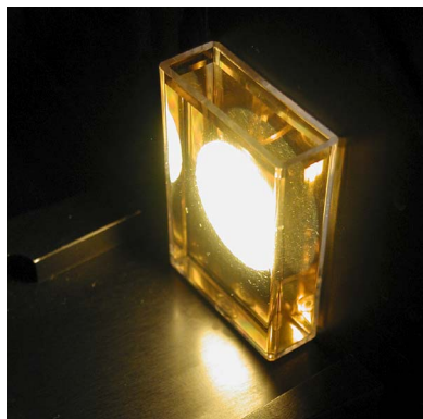
10-mm Acrylic Cell on standard C02-1005-481 Transmission Cell Holder measuring transparent liquids in TTRAN mode
