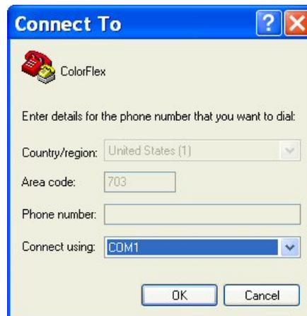
8. On the Connect To screen, indicate which of your computer's communications ports is being used for the instrument connection. Then click **OK**.
