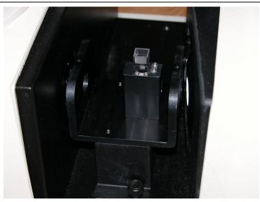
Cautions: The same cell used to hold the blank during standardization should be used for sample measurements, particularly when disposable cells are used.
