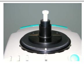
Cautions: Variable sample illumination (VSI) option required. The powder holder should be used ONLY for color difference measurements.
