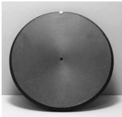
*Cautions: Variable sample illumination (VSI) option required. Performance specifications will not be met with this smaller-than-standard port plate. The change of geometry with this option will cause a slight shift in the color values of the calibration standards.*
