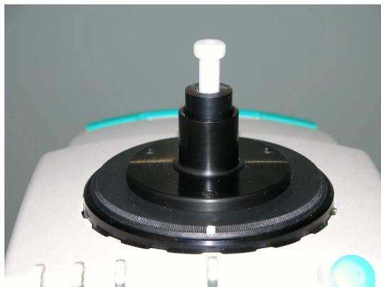
*Cautions: Variable sample illumination (VSI) option required. The powder holder should be used ONLY for color difference measurements.*
