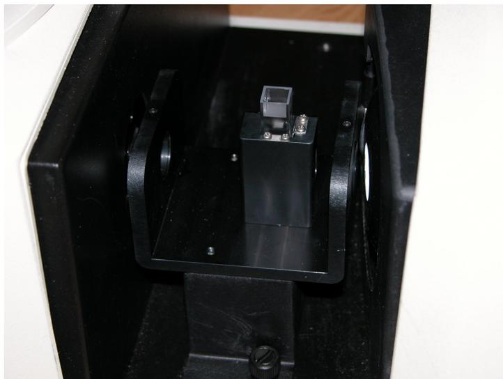
*Cautions: The same cell used to hold the blank during standardization should be used for sample measurements, particularly when disposable cells are used.*
