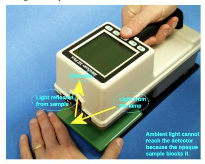
**Transparent samples** (such as clear liquids and clear glass) transmit all the light from the source lamp to the instrument's detector. Generally, no light is lost to reflection, though ambient light may be transmitted to the detector along with the light from the source lamp. This ambient light could potentially affect the color measurement, as the amount of light transmitted to the detector is increased.
