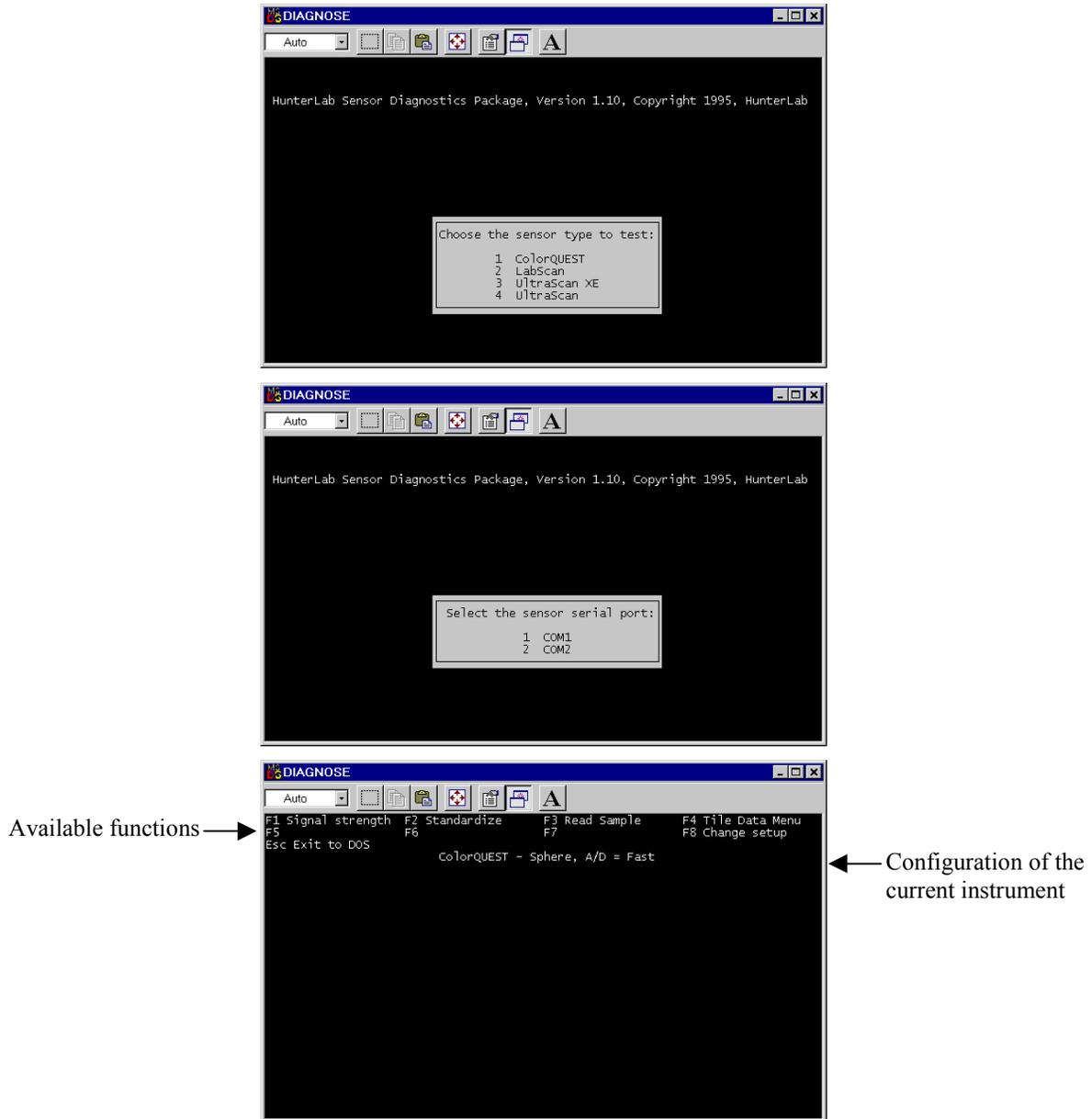
5. Place the white calibrated tile at the reflectance port. Press **F1** to perform the **Signal strength test**. The raw A/D counts for the white tile are then displayed for each measurement wavelength. The highest A/D value shown should be between 32,768 and 45,875. Press Home to exit the menu.
