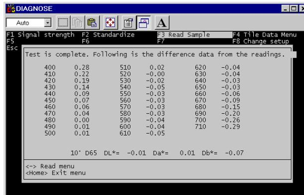
11. Press F4 to display the **white and gray tile data** stored in the instrument. Press 1 to display the RSIN data and then Home to exit to the diagnostics menu.
