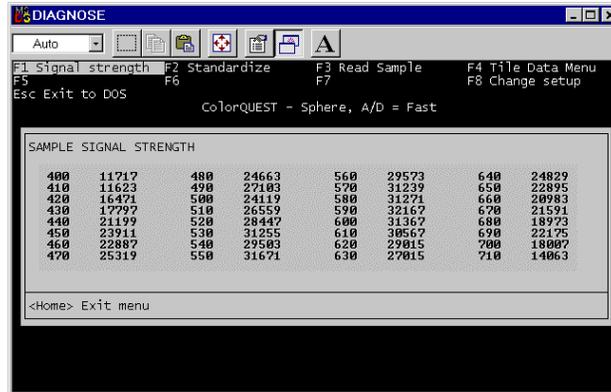
6. Place the black card over the lens in the transmission compartment and press **F1** again. All of the A/D values should be between 655 and 2,621. Press Home to exit the menu.
