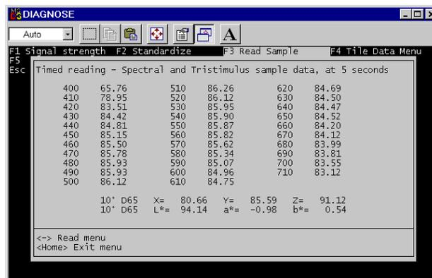
9. Press 2 to perform the repeatability test. Place the white calibrated tile at the reflectance port. Press Insert. Twenty reads of the tile will commence and Delta L\*, a\*, and b\* values (between the first and last readings) will be displayed on the screen along with delta values for reflectance at each wavelength read. If any of the spectral value deltas is outside the following specifications, record the result and contact HunterLab Customer Support.
