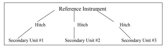
Here's a simple example: A MiniScan XE Plus was used to read a green standard and a green sample. It was then hitched to the green standard values read on another instrument and the green sample was read again. The values read on the MiniScan XE Plus are shown below.
