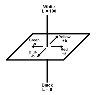
There are delta values ( $\Delta L$ ,  $\Delta a$ , and  $\Delta b$ ) associated with this color scale. These values indicate how much a standard and sample differ from one another in L, a, and b. The  $\Delta L$ ,  $\Delta a$ , and  $\Delta b$
