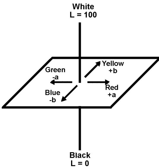
There are delta values ( $\Delta L$ ,  $\Delta a$ , and  $\Delta b$ ) associated with this color scale. These values indicate how much a standard and sample differ from one another in L, a, and b. The  $\Delta L$ ,  $\Delta a$ , and  $\Delta b$
