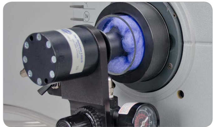
Figure 2. Compression Cell for pressing loose fiber flush against a sample cup window, minimizing light trapping by the loose fiber.
