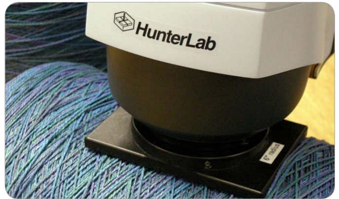
Figure 1. MiniScan EZ with bobbin adapter to consistently place the instrument flush on the curved surface of a textile cone or bobbin.
