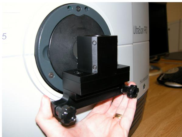
4. Tighten the holder into place by turning both knobs clockwise.
