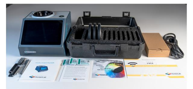
ColorFlex L2 Instrument • Standards Case • Diagnostic Check Tile (Green Tile) • Instrument Standard (White Tile)
