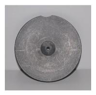
**Installation:** To install the port plate, remove the standard port plate and snap the modified port plate into place at the reflectance port.
