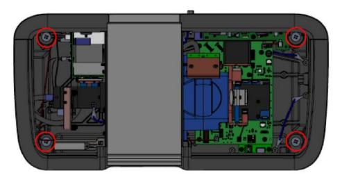
5. Remove the Front and Rear covers by removing the 4 screws inside the instrument as shown below.
