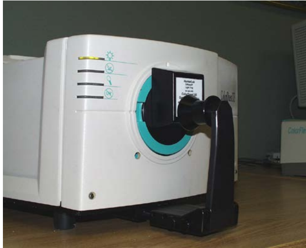
Standardizing on the light trap
