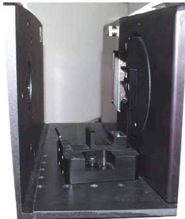
Transmission clamp as placed in the transmission compartment for measurements in total transmission. The clamp is placed flat at the sphere.
