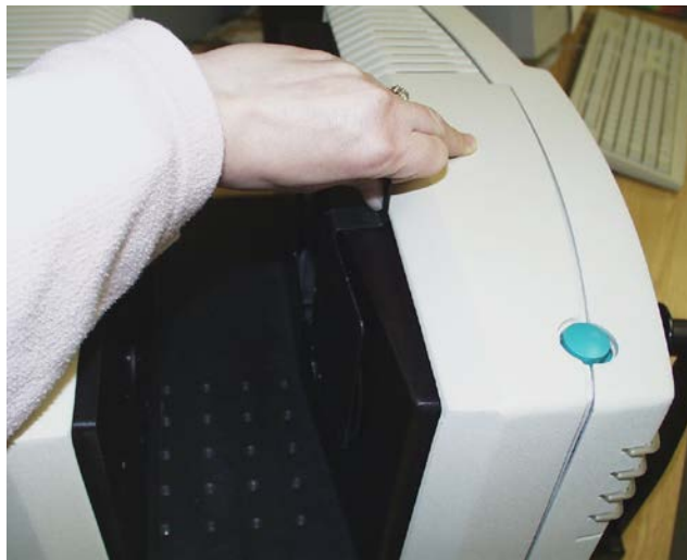
Standardizing on the black card device for TTRAN mode. (The transmission compartment door may be closed down to the device handle.)
