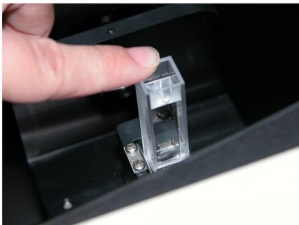
4. Complete the standardization by measuring the cell blank as the top of scale.
