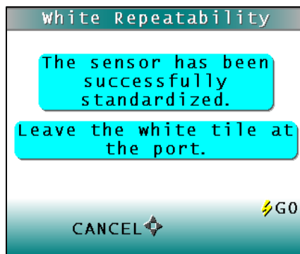
Figure 100. Initiation of Repeatability Test
