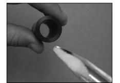
2. Pack the powder down using the plunger. Do not overtighten the powder holder. The powder should be at least 1/2-cm deep in the holder.
