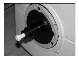
Note: The powder holder should be used ONLY for color difference measurements.
