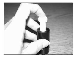
3. Place the powder holder into the port plate and measure the sample.
