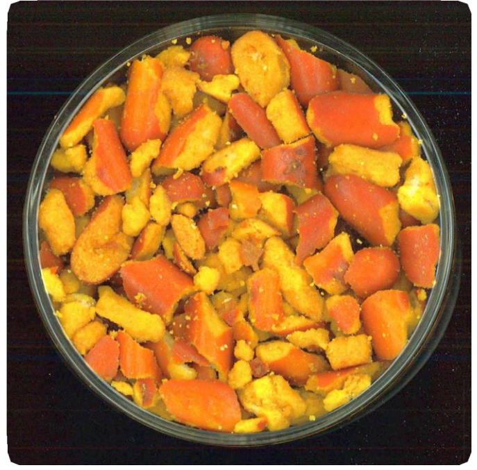
This is the instrument view through the bottom of the dish. The instrument optically averages all colors within the field of sample view.
