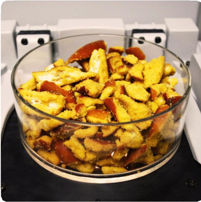
Glass sample cup with pretzel bites ready for color measurement on a HunterLab Aeros with a large diameter area of sample view.
