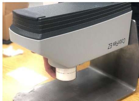
Figure 3. Port-Down Sample Measurement
