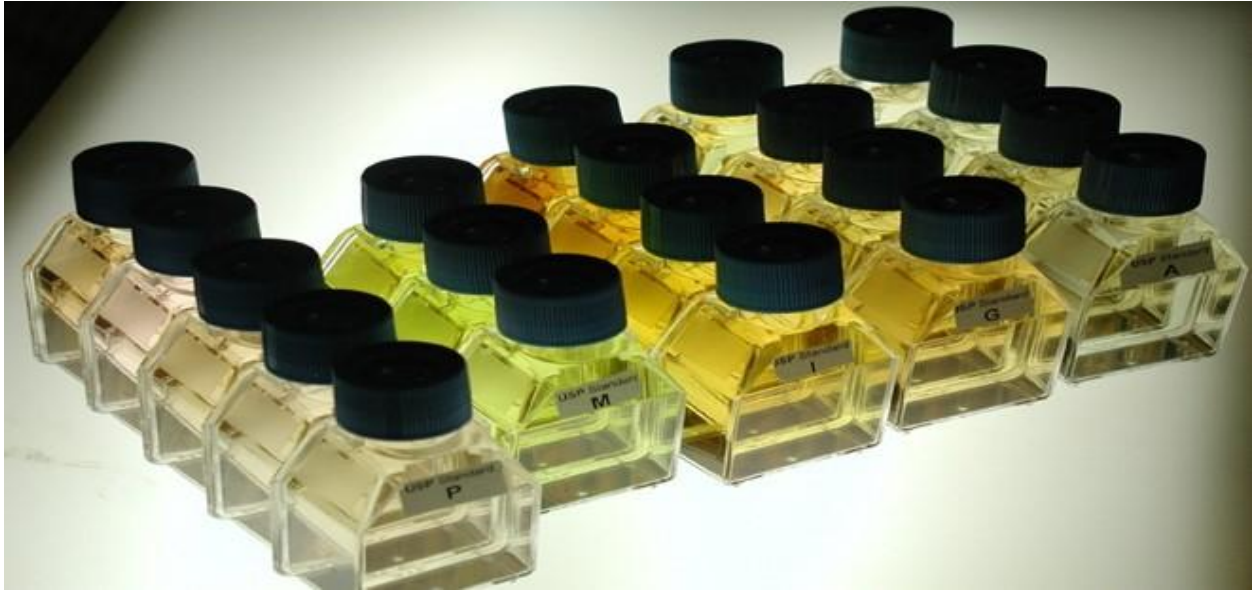
Figure: Example of USP pharmacopeial liquid color standards (15 standards designated A-T) in vials with controlled illumination and background.
