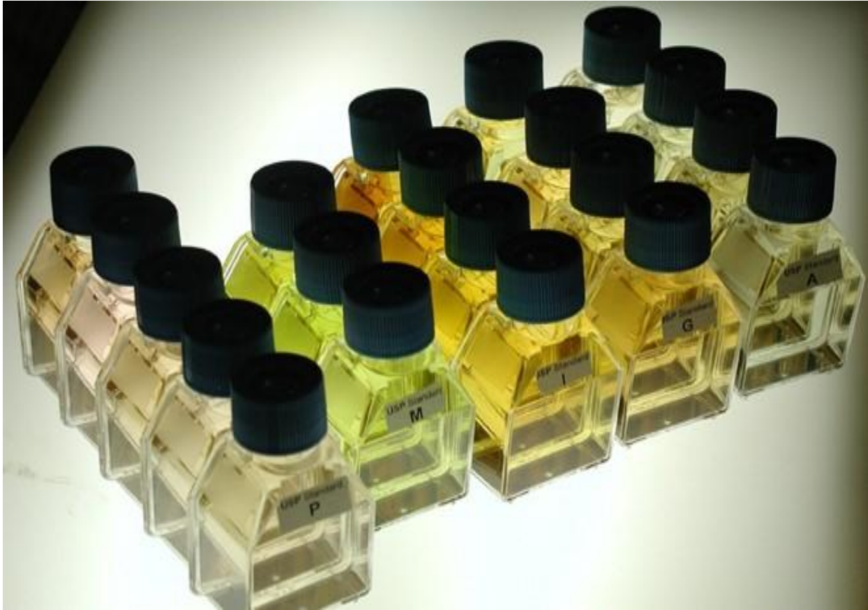
Figure: Example of USP pharmacopeial liquid color standards (15 standards designated A-T) in vials with controlled illumination and background.
