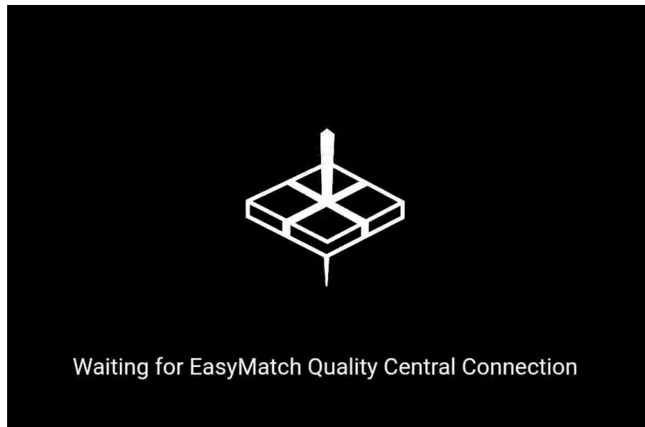
Figure 20. Essentials L2 Waiting Screen — Local Measurement Disabled
