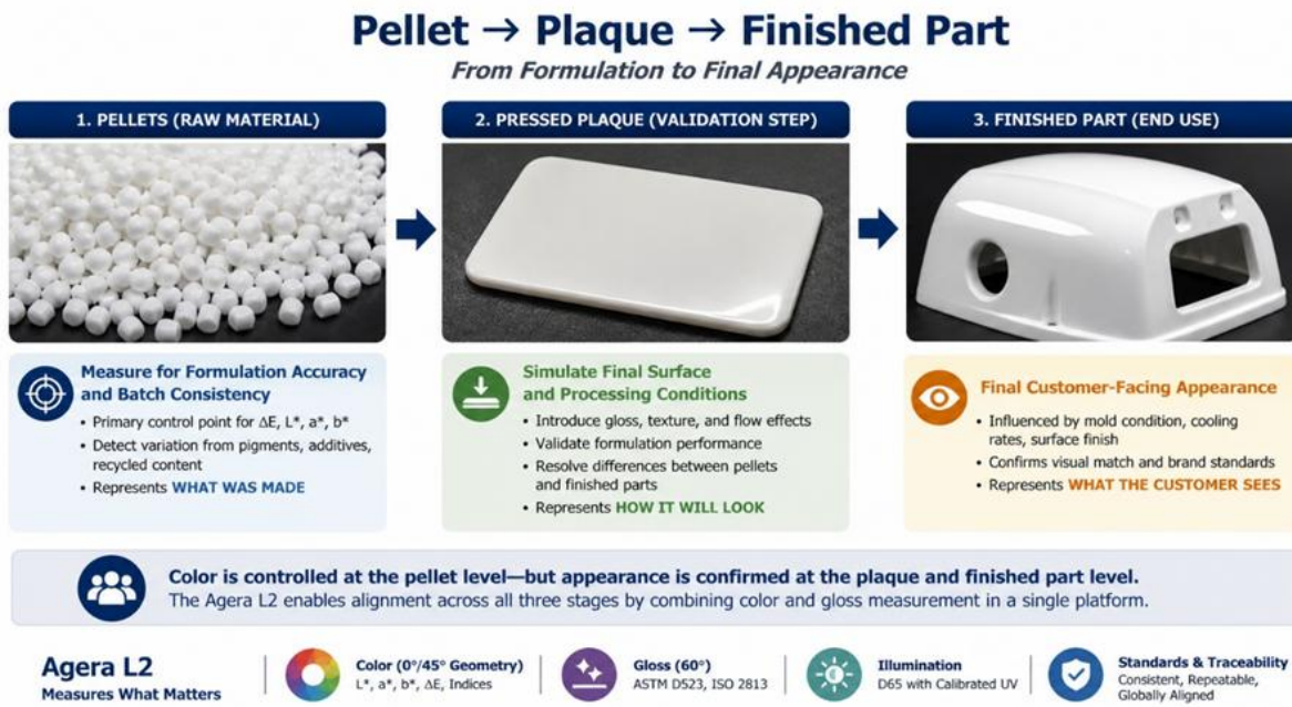
Fig. 1: Pellets define the formulation—but plaques define the appearance. Gloss measurement bridges the gap between the two.
