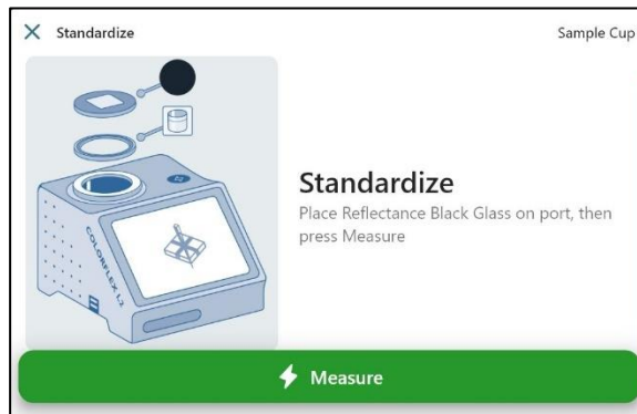
Figure 2. Measure Reflectance Black Glass
