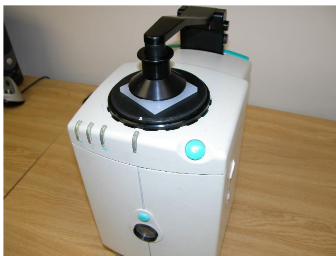
Figure 26. Sample Clamp in Port-Up Position
