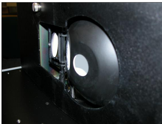
Figure 6. Specular Exclusion Port Open
