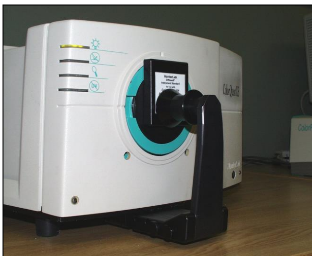
Figure 15. Setting Top-of-Scale with the White Tile
