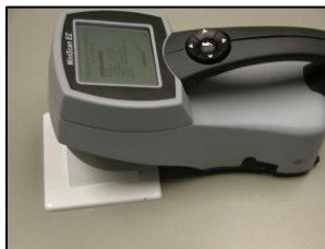
Figure 66. Using a White Tile Backing
