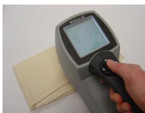
Figure 64. Measuring Thin, Soft Materials
