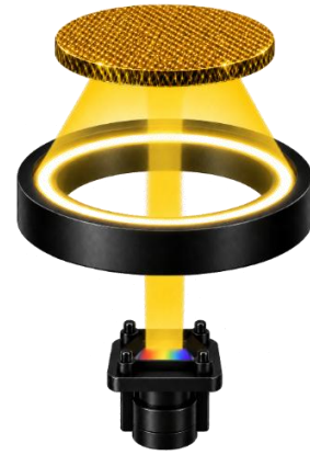
Image 5: 45^\circ annular illumination \rightarrow 0^\circ viewing
